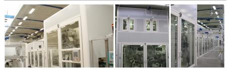
A new machine for the production of adult incontinence pads from an Italian supplier had to comply with the Danish requirement of a noise level of 80 dB(A). The acoustic enclosure also had to serve as a safety guard as well as meet requirements for visibility and easy accessibility. IAC Nordic supplied an acoustic enclosure comprising many doors and large glass panels. This reduced the noise level from over 100 dB(A) to under 80 dB(A) in all measuring points.
